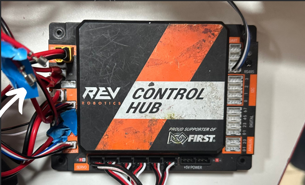
the broken port
